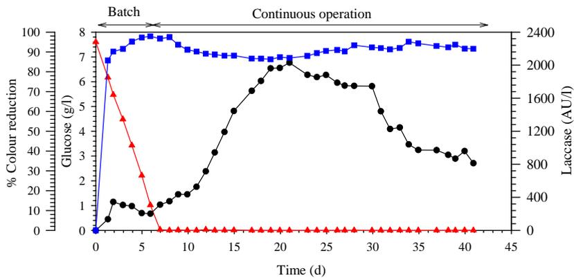
Fig. 2. Glucose concentration (▲), laccase activity (●) and percentage of colour removal (■) during the continuous biodegradation of the dye Grey Lanaset G by *Trametes versicolor*.
